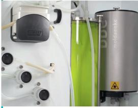
Sample water is mixed with the algae test olution and then analysed.
