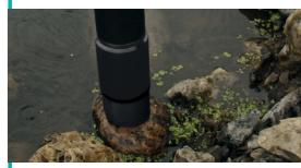
The BenthoTorch used to measure algal classes and their concentration on a stone surface.
